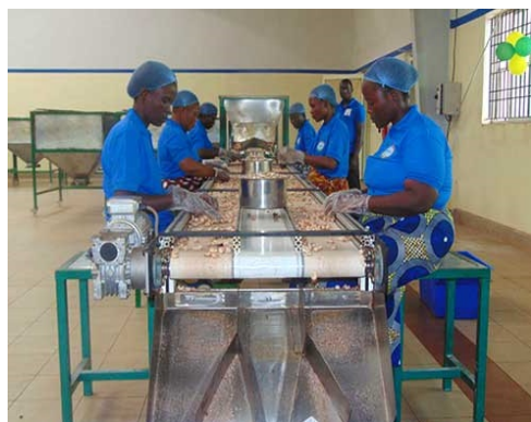
Workers inspect cashew nuts for quality in Fludor cashew processing facility, which balances automation with manual labor. Credit: USDA
